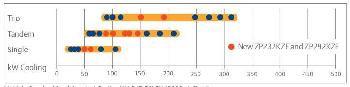
Multiple Copeland Scroll Nominal Cooling kW @ (5/50) EN 12900 - 1 Circuit
